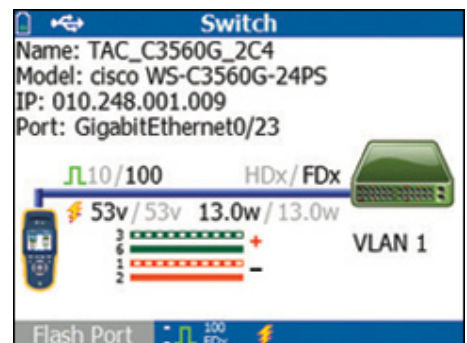
100 Mbps link on copper with PoE on port 23
